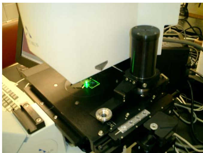
Fig. 5: Using fluorescence for IF-IHC-stained sections during LCM.
