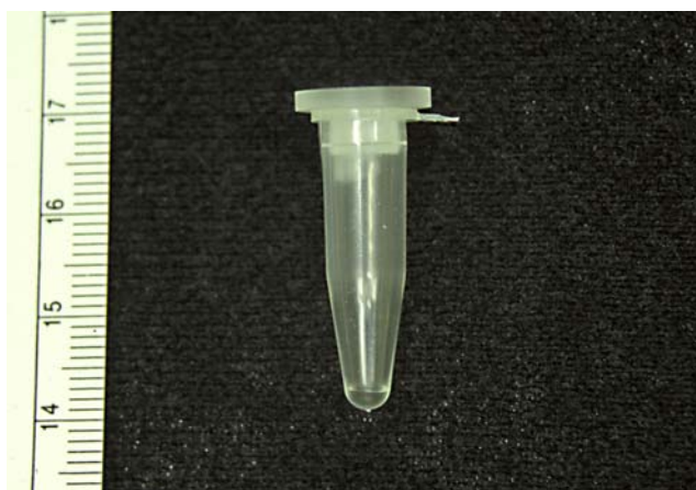
Fig. 22: The ABI 0.5 mL GeneAmp tube containing 10 uL Lysis Buffer.
