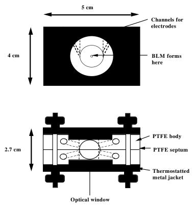
Figure 1. A Schematic diagram of the cell developed for formation of planar lipid bilayers (PLBs) for combined optical and electrical measurements
