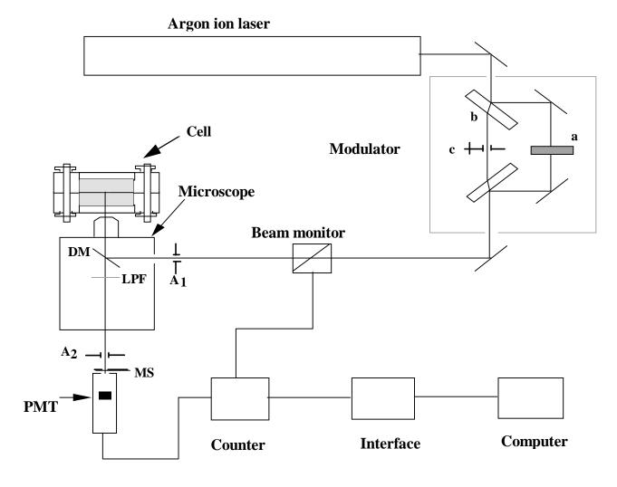
Figure 2. Schematic diagram of the principal components of the Fluorescence Photobleaching (FRAP) apparatus
