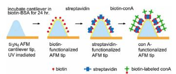
Fig. 2: Functionalization of an AFM tip with concavalin A. Unsharpened  $Si_3N_4$  AFM cantilevers were functionalized with biotinylated bovine serum albumin (biotin-BSA) coupled with avidin bound to biotinylated conA.
