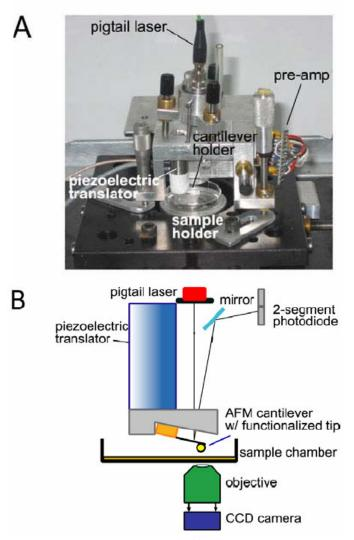
Fig. 1: (A) Photograph of our AFM set-up. The CCD camera is not in view. (B) Complete schematic diagram of the AFM.
