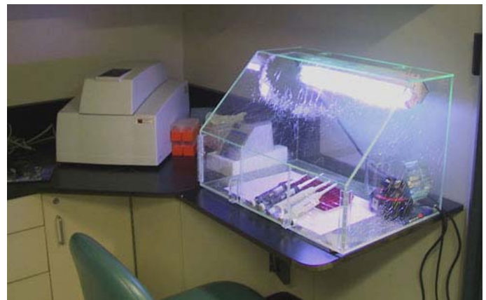
Fig. 6: UV-equipped Plexiglas hood is used in order to prevent sample contamination.
